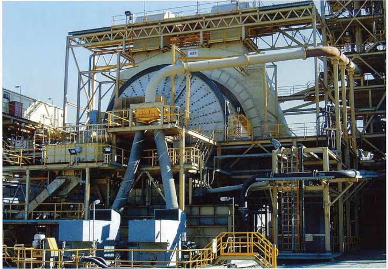
The Lefroy mill's centrepiece is the 11m-diameter SAG mill, which utilises an advanced multi-variable control system.
